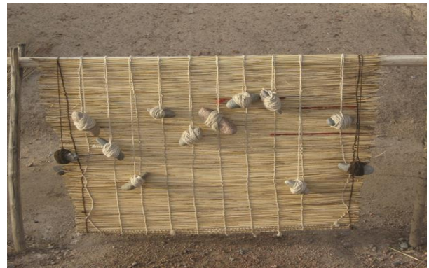
straightening wool cords with stones for preparing traditional canvas (photo by Rahimov Ruslan)
